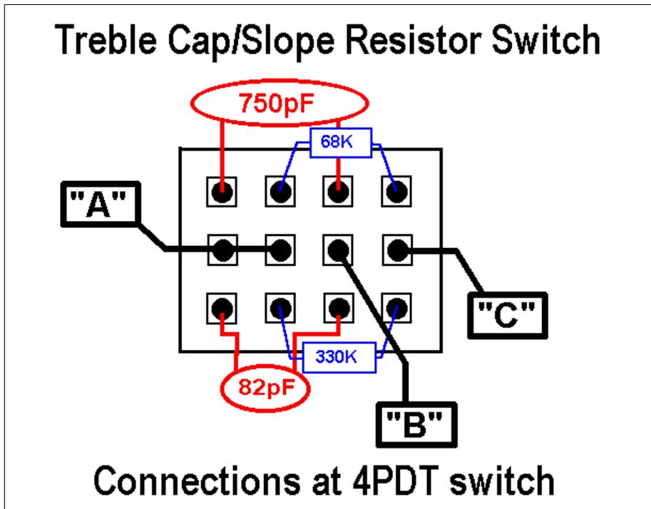
Diagram 2 for advanced treble cap/slope resistor mod:
