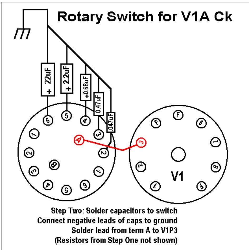
Diagram 1 for advanced treble cap/slope resistor mod:
