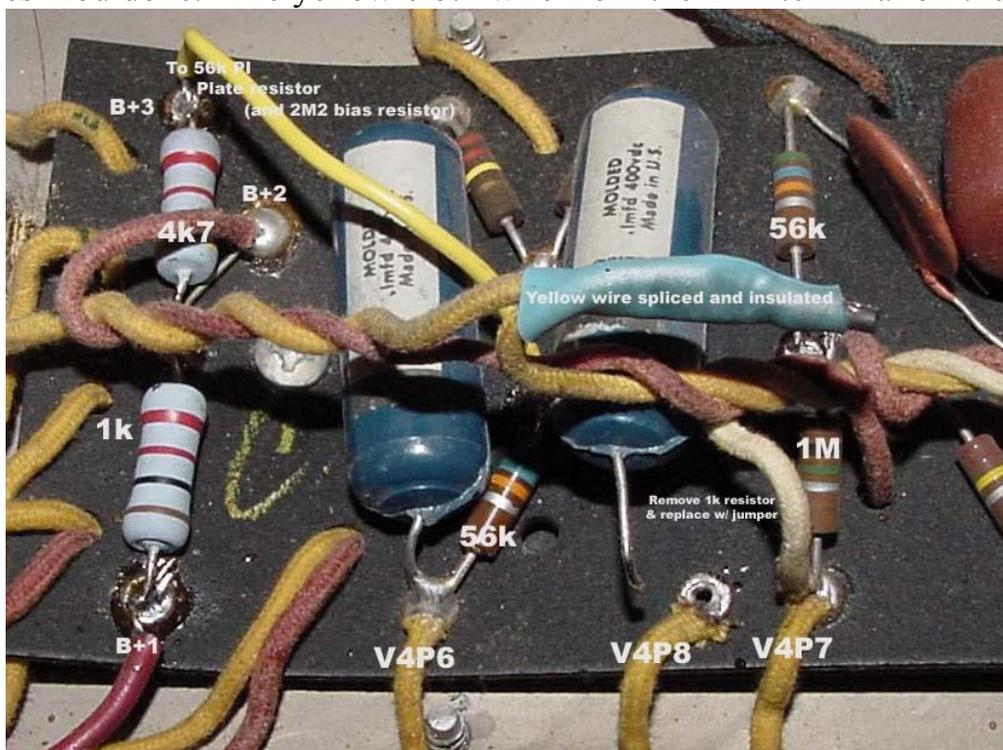
The Rick E. mod has already been completed, with me replacing the first two power supply resistors with metal oxide resistors. The first resistor is the 1K resistive choke; the second resistor (18k) was replaced with a 4.7k resistor to lower the voltage drop between B+2 and B+3.
