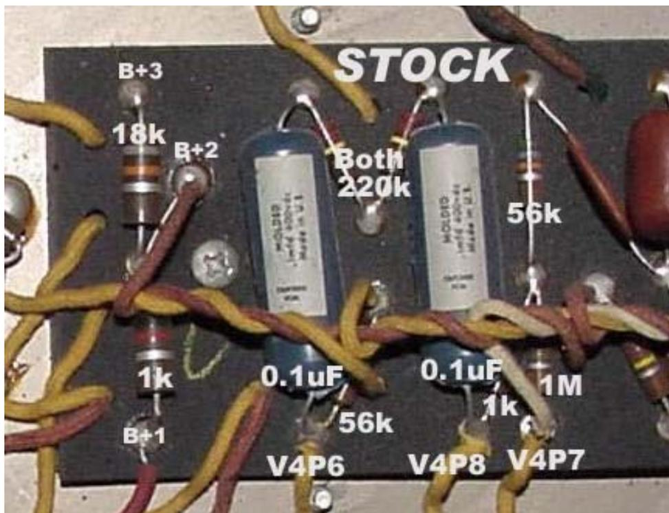
The picture to the left shows the phase inverter for my 1964 Princeton Reverb, with all of the basic components labeled. The picture to
