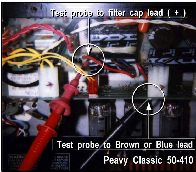
**Figure 4. Measuring idle bias current**
