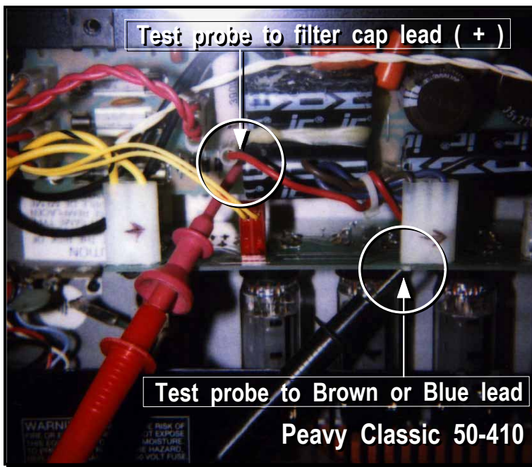
Figure 4. Measuring idle bias current
