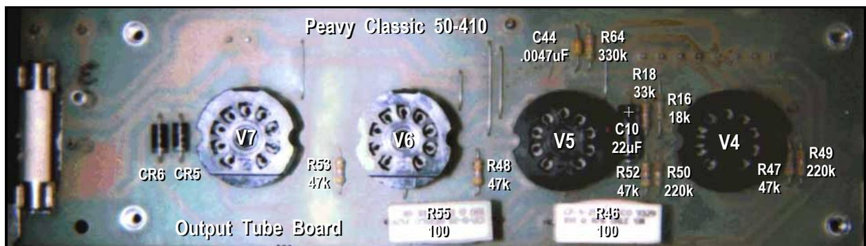
Figure 1. Components on the output tube board
