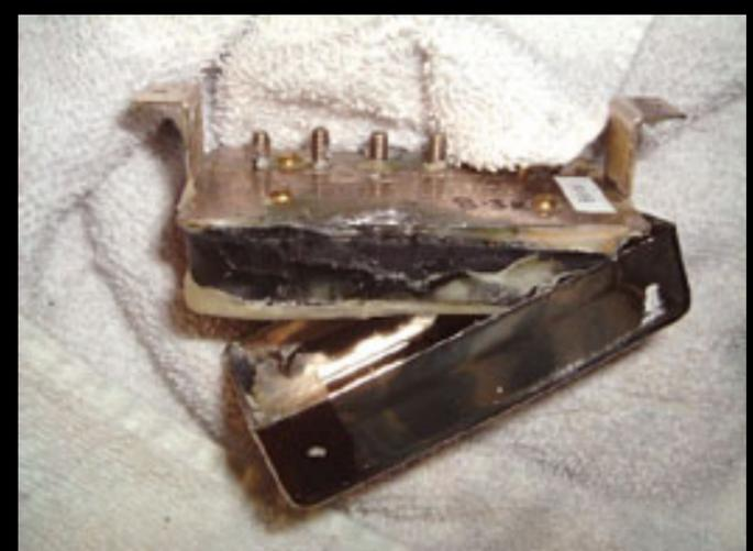
**Step 7** Loosen only, the 4 very small sized Philips screws on the bottom plate of the pickup
