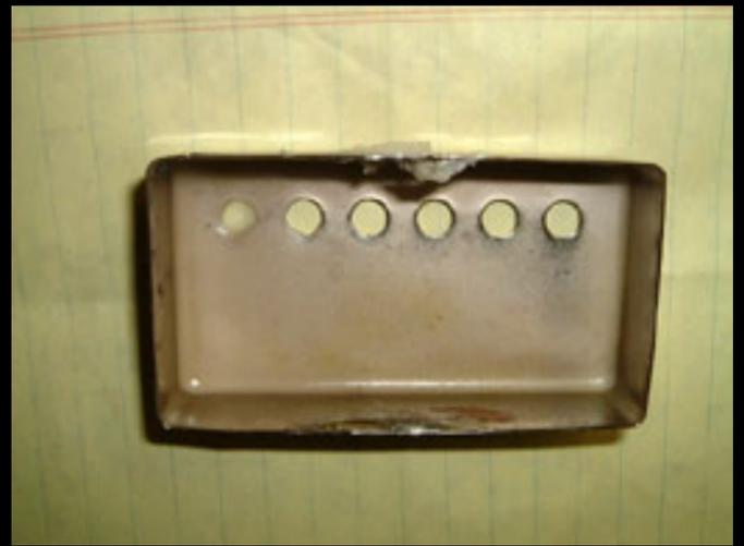
**Step 14** Press the cover on as far as you can first with your fingers, feeling for the cover bottoming out onto the pickup top.
