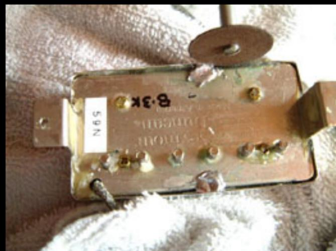
**Step 5** Take a Dremel tool with a thin cutting wheel on it and cut through the solder on both sides of the bottom plate to have the ability to remove the cover shortly Try to cut the solder right between the cover and the base plate.
