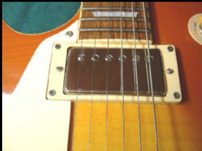
This is a Seymour Duncan 59 Neck Pickup that I want to exchange an A3 bar magnet with an A5. I want chimier highs, overall tighter pickup response and tighter lows, less mid. This pickup has a nickel cover which has to be removed for access to the bar magnet.
