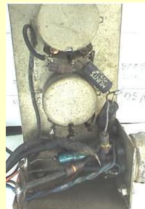
Rear view of an original JMI "Brilliance" unit. It consisted of an 'L' shaped bracket, with a 12AX7 mounted sideways, & the two tone pots facing the rear. A white labelled fascia plate was also included
