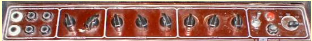
A 1963 Copper control panel with integral Topboost. The existing jacks and controls were squeezed together to make room, and the Treble & Bass controls were added alongside the Tone Cut Control. Inside, the extra 12AX7 was added to the preamp section of the chassis. Only the addition of a Standby switch and the small JMI logo distinguishes this from the current AC30TB
