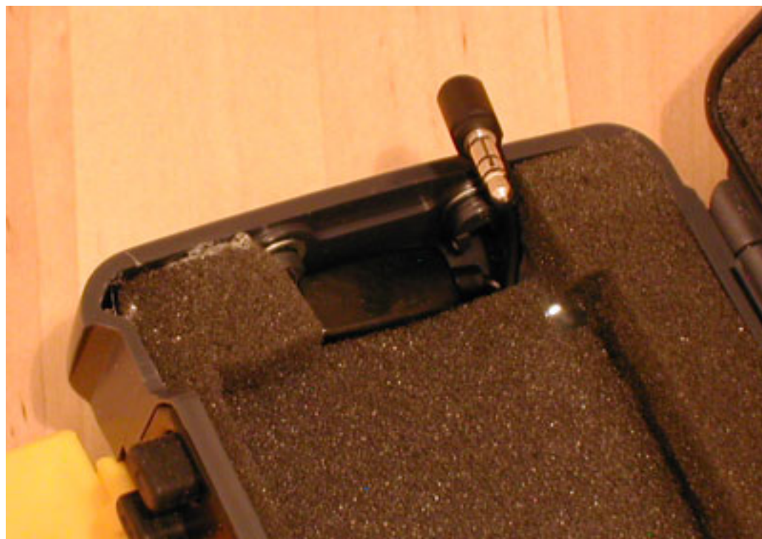
Closeup of the internal headphone jack. The black piece between the foam and the side of the case is the volume control. The external headphone jack is to the right of the volume control and hidden under the foam. To prevent the possibility of a short, the solder joints on the external headphone jack were coated with hot glue.
