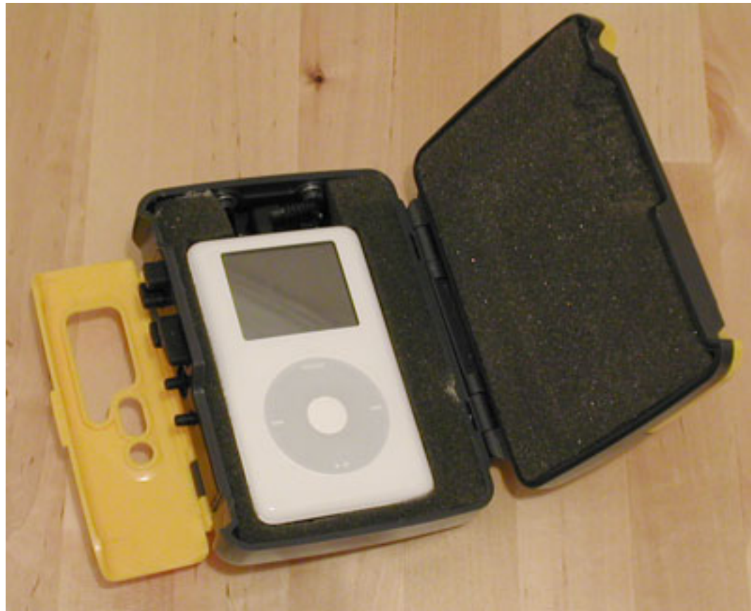
The final product. Note the cutout in the foam on the lid to allow the case to close properly.
